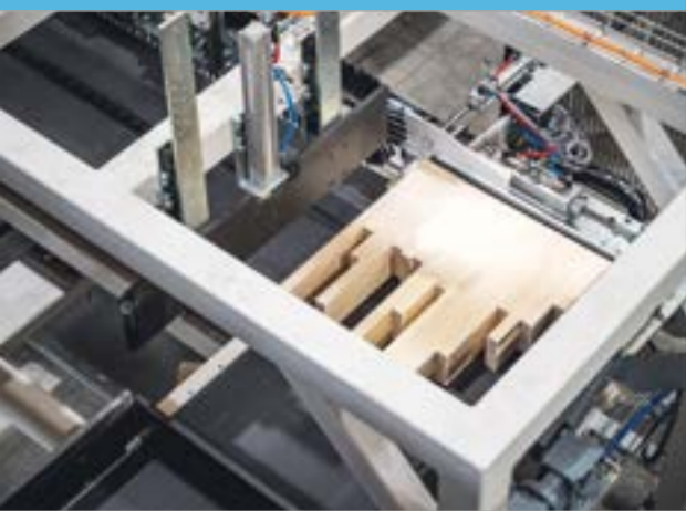
The System TM batch builder creates batches of 600-millimeter width.
